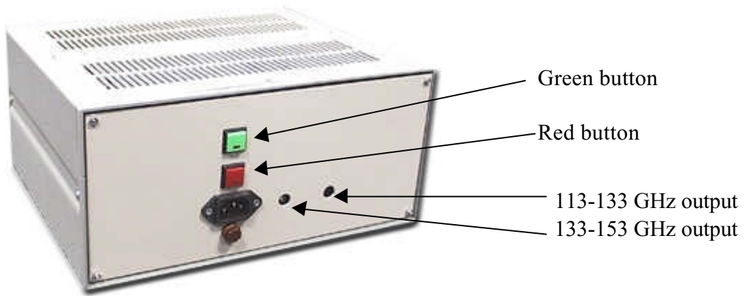
Fig. 6. Outward appearance of the RF Block.
