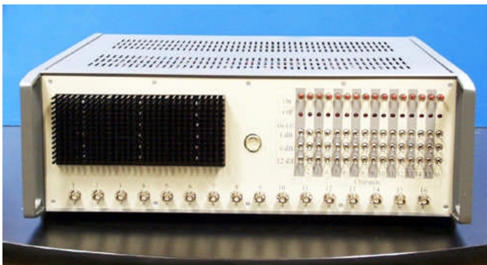
Fig. 10. Outward appearance of the IF Block.
