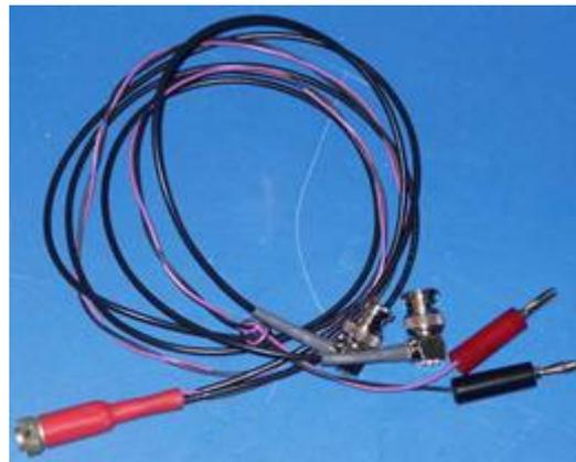
6. Connect pin connectors (red – signal, black - common) of special cable to DC voltmeter. Estimated voltage range measurement  $< +10\text{DCV}$ . BNC connectors to any oscilloscope for control 50 kHz IF signals.
